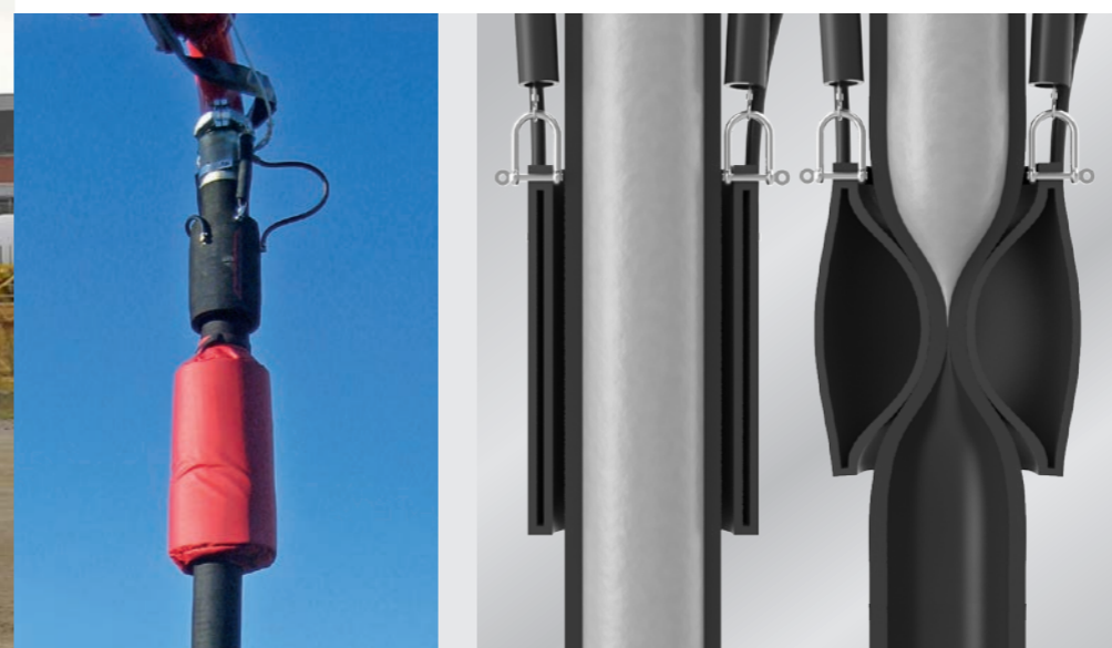
In comparison to the 47-5, the 46-5 has less horizontal reach but allows a higher boom tip load. This means that an end hose squeeze valve (EQV) and a divided end hose can be used.
